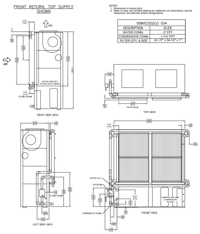
Fig. 13 — 50BVC, J, Q034 with Optional Waterside Economizer Dimensions
